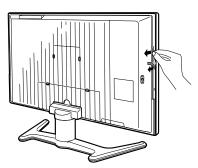
Peel off the tape holding the ends of the cables, and move cables towards behind the display.
